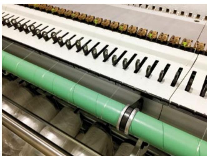
*The perfect timing between the yarn feed system and the embroidery frame movement, enables the flawless embroidery quality to be achieved. The thread is fed depending on the pattern design, stitch length and weaving speed. It ensures that, all different thread types are fed properly. the thread feeding system, yields quick and easy thread replacement while providing excellent thread retention.*
