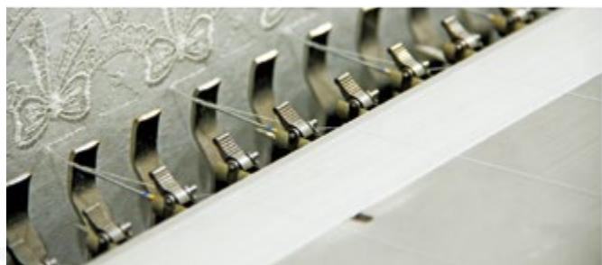
*Thanks to lightweight mass of moving parts in our design, direct drive fabric presser touch angles and timings are electronically controlled in order to prevent pattern distortions over embroidery. This silent, low energy and maintenance free system allows the user to make the desired adjustment to achieve perfect embroidery quality.*
