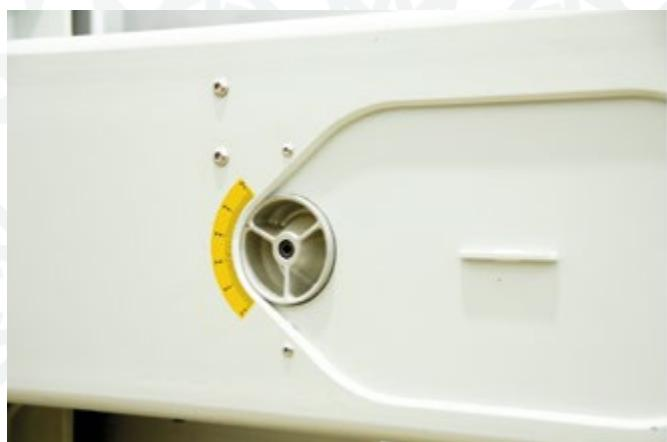
*An excellent embroidery quality can be achieved by use of adjustable shuttle box position according to needle. Shuttle box position can easily and quickly be adjusted as small as 0,1 mm precision at any time either the machine running or stopped.*
