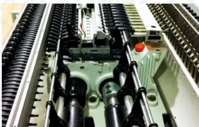
*Due to the multi-point drive system, the weight of the oscillating parts is reduced, ensuring efficient, precise, quiet and vibration-free working conditions at high speeds. The motion is transferred directly to the needle/bohrer spindles and thread guide. Needles and bohrers, are driven by the same cam. By means of pneumatic driven selector mechanism, the needles and bohrers can be selected automatically thus extensive machine operation is guaranteed.*
